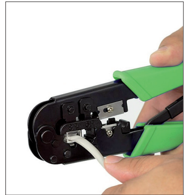
Crimp the connector and make sure that it is securely fastened.
